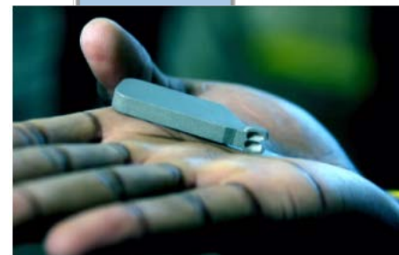
Additively Manufactured Pelton Buckets
