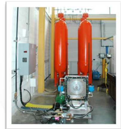
GLIDES first-generation proof-of-concept 1.5-3 kW prototype
